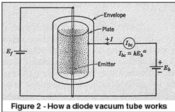
Figure 2 - How a diode vacuum tube works
